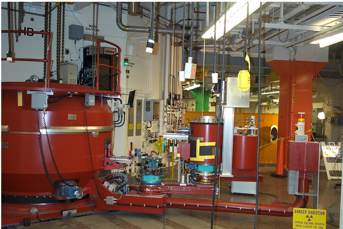
Figure 2: HB-1 Triple Axis Spectrometer Instrument
